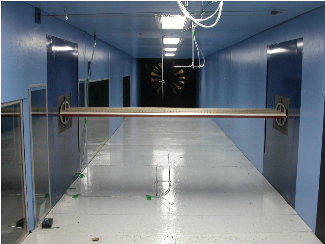
Figure A-2: Sectional Models in RWDI's Boundary Layer Wind Tunnels
